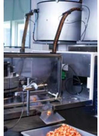
*The photo shows a machine for Ø 20 mm capsules. Capacity: 400 units per minute.*
