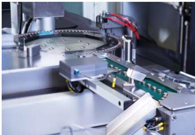
*Machines equipped with two star wheels are provided with a vision system checking the rubber for possible defects inside the capsule.*
